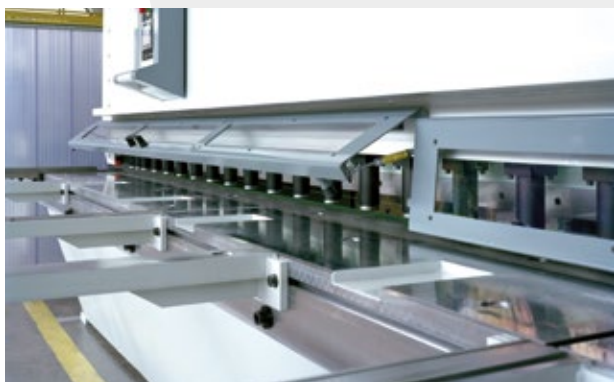
Paramani ribaltabile. Movable swing-up front safety guard.
