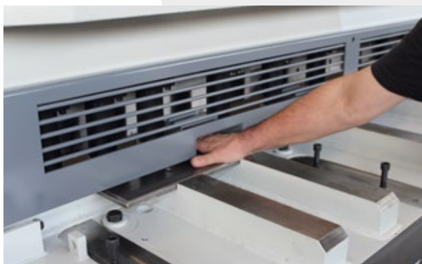
Paramani a greca. Shaped front safety guard.
