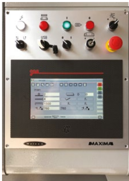
CNC ESA VIS-630 a 4 assi touch screen 10" CNC ESA VIS-630 up to 4 axes touch screen 10"
