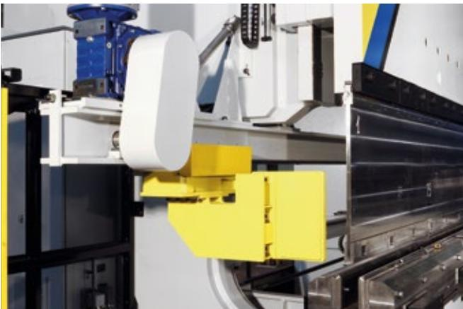
The motorized extractor is a device that assists with the removal of formed parts from the lateral side of the machine, ideal for the production of long poles and polygonal shaped parts.
