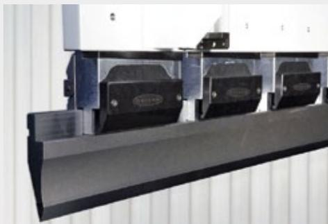
With the pneumatic tool clamping system WTC, patented by Warcom, all PROMECAM tooling up to 20 Kg can be loaded from the front side.
