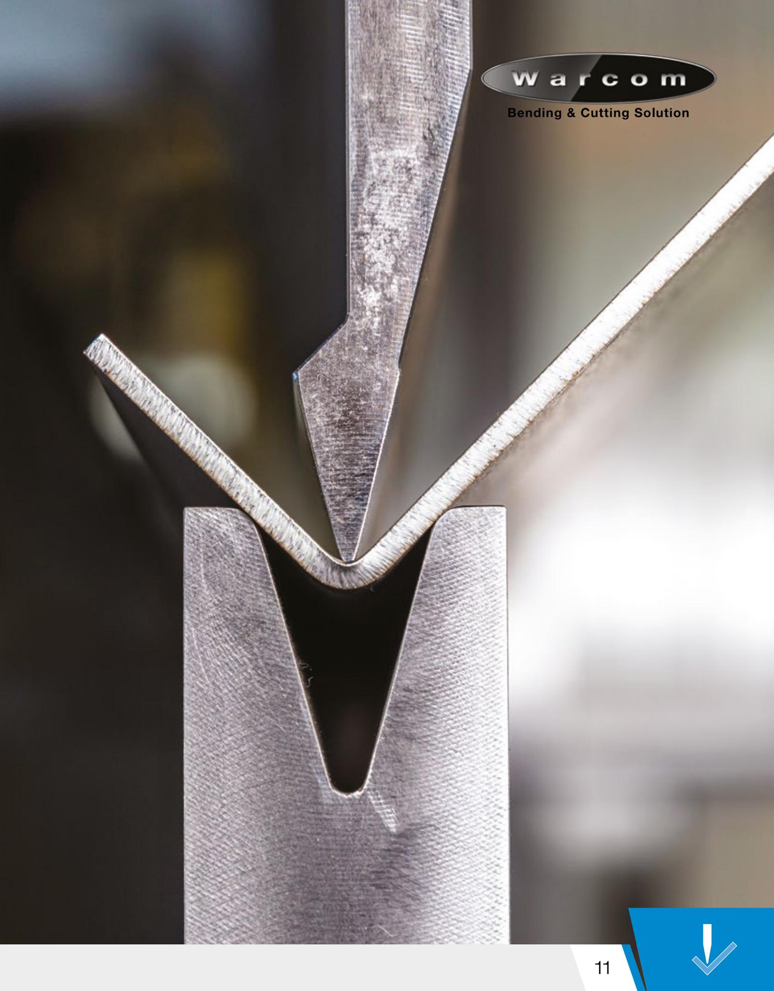
A close-up photograph of a metal bending process. A vertical metal strip is being bent by a V-shaped die. The metal strip is positioned above the die, and its edges are being forced into the die's V-shape. The metal has a textured, brushed appearance. The background is dark and out of focus.
